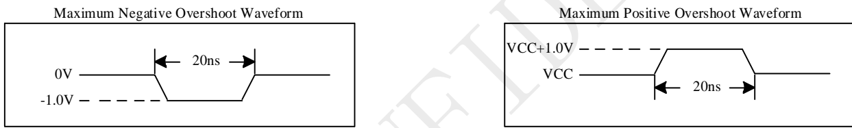
Figure 5-2 Input Test Waveforms and Measurement Level
